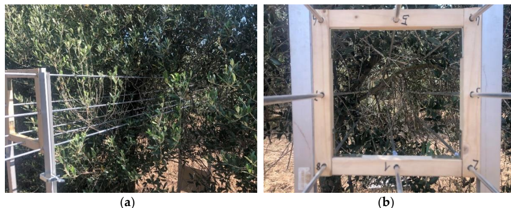
Figure 2. (a) Canopy interceptor with the bases positioned on the two sides of the olive hedgerow. The frame helps to select a 25 \times 25 \text{ cm} area while the long rods delimit the volume of the canopy to be sampled; (b) intercepted volume of the canopy. Only the bare shoots are visible after the detachment of all the leaves
