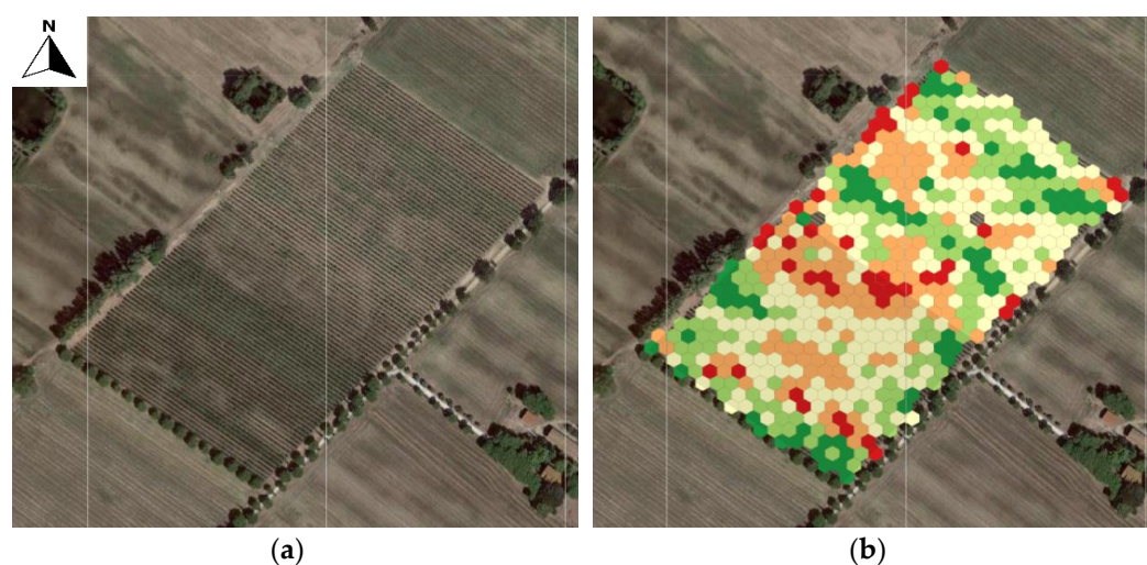
Figure 1. (a) Satellite image of the rectangular olive orchard interested by this study; (b) map of the same orchard with area points of different color based on NDVI data from satellite observation. Each color is related to the class of relative NDVI index: red = very low, orange = low, yellow = middle, light green = high, dark green = very high.
